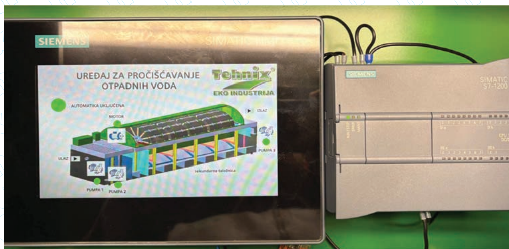
HMI panel i PLC uređaj
