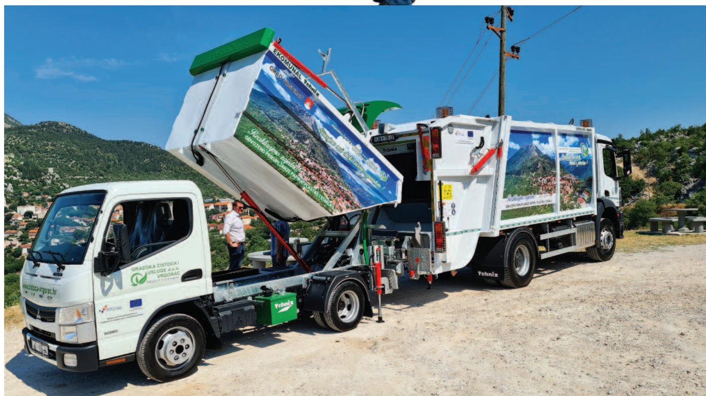
POSSIBILITY OF RELOADING FROM SMALL TO LARGE VEHICLES USING HYDRAULIC
