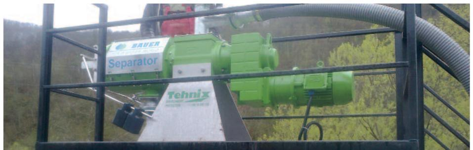
SLUDGE SEPARATOR FOR BIOREACTORS AND FARMS
