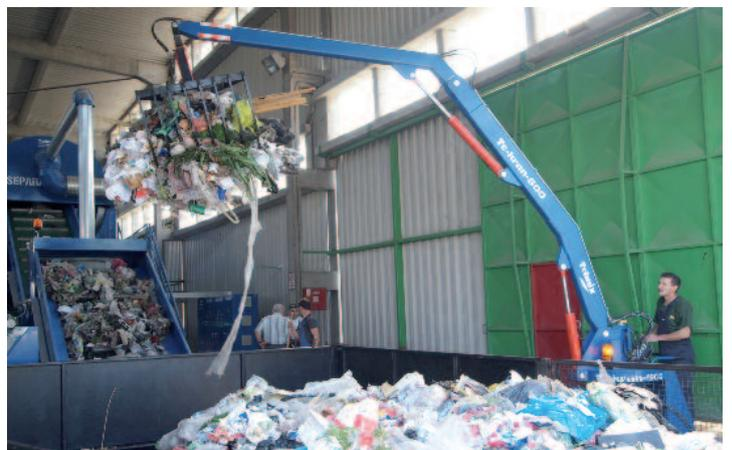
TEKRAN TEHNIX - for dosing of mixed communal waste
