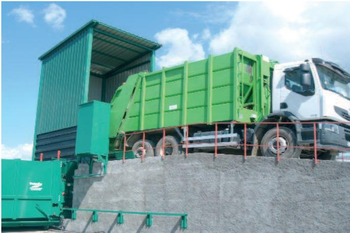
Automatic reloading station type Tehnix - from garbage truck to 32 m<sup>3</sup> press-containers
