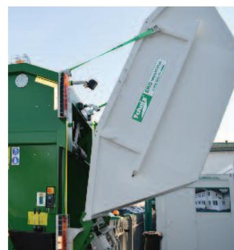
Automatic discharge of receiving chamber inside and outside the cabin
