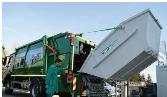
Tehnix skip loader for containers 5 and 7 m<sup>3</sup>
