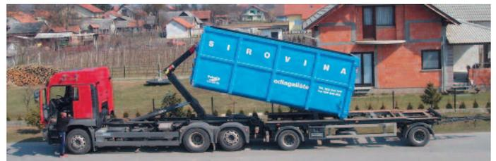
Fast cargo discharge and loading, practical exchange - full for empty
